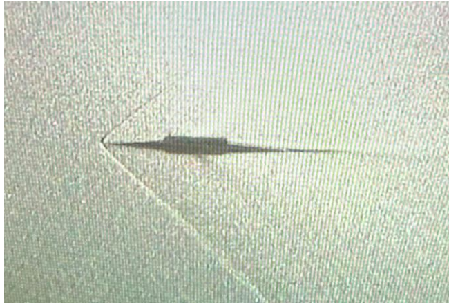
Figure 3: A photo of the Schlieren visualization of the 10-degree wedge at 0 degrees. The image is flipped vertically to show the true top, rather than the upside-down Schlieren-reversed image.
