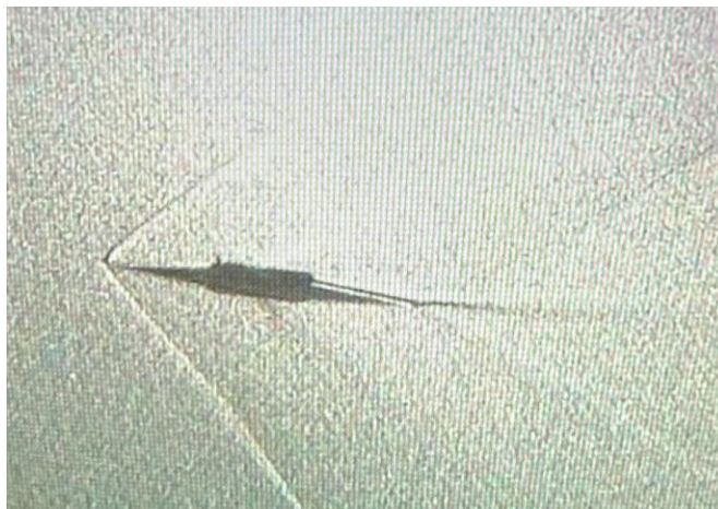
Figure 4: A photo of the Schlieren visualization of the 10-degree wedge at 2.5 degrees counter-clockwise turn. The image is flipped vertically to show the true top, rather than the upside-down Schlieren-reversed image.
